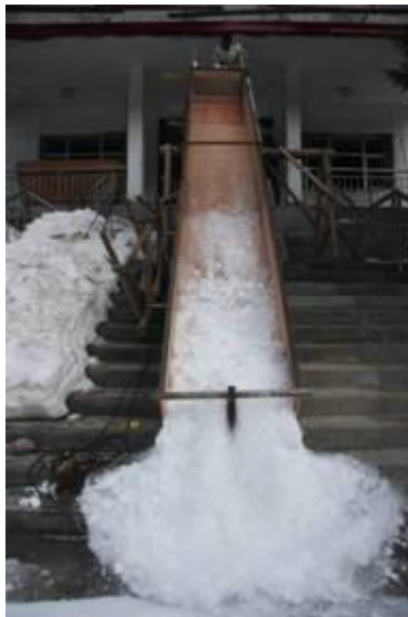
Fig.3.9 Avalanche testing system (adapted from Tianshan Snow-cover & Avalanche Research Station, CAS home page)
