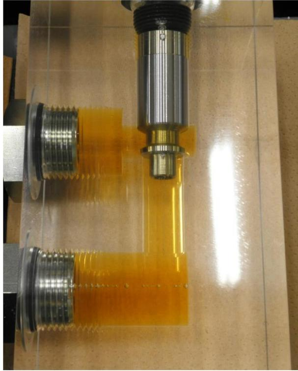
Figure 2-3 Photograph of tested poppet valve
