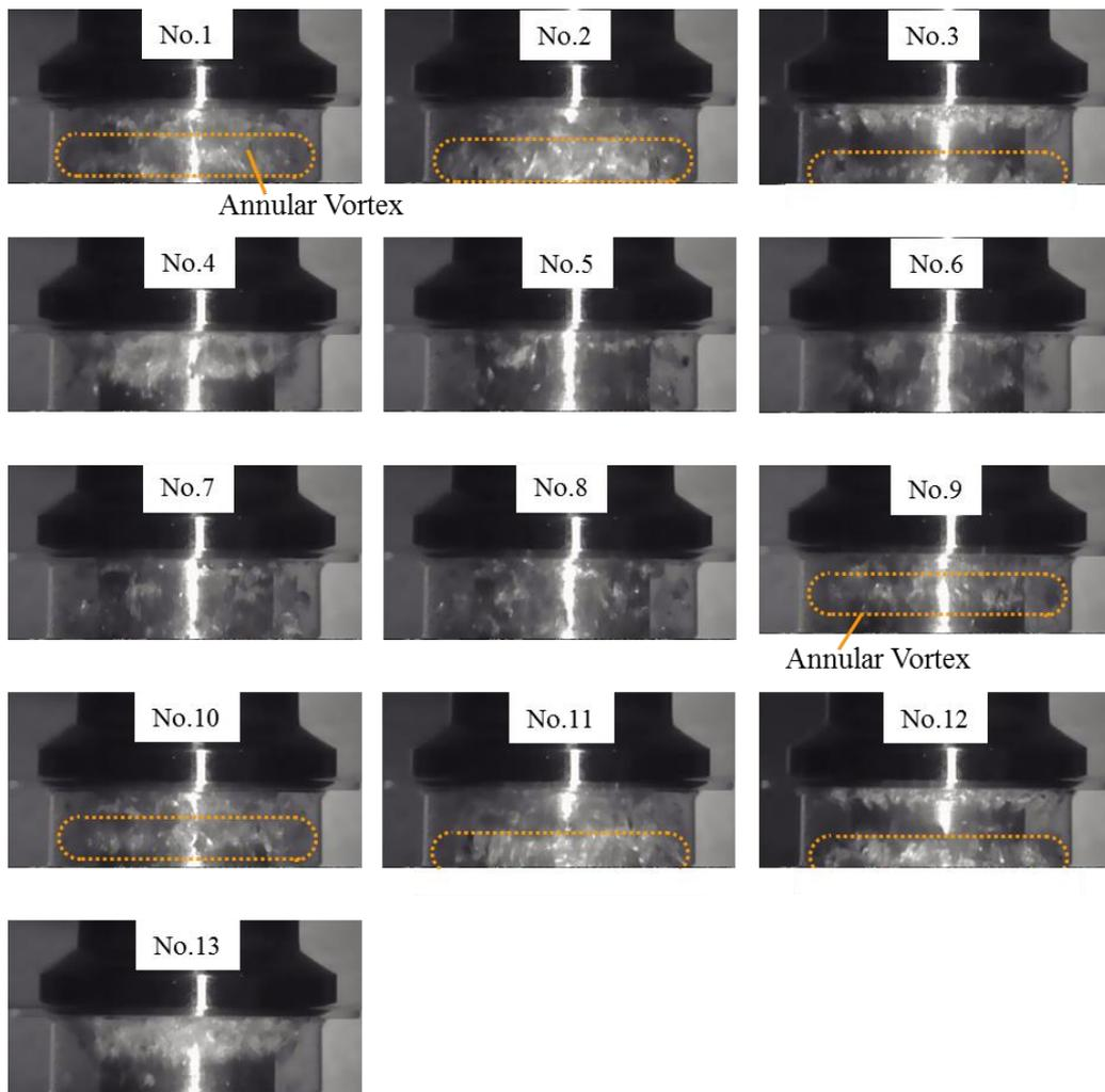
Figure 4-8 Transient state of cavitation for  $Q_{pump} = 20$  L/min and  $T = 40$  °C.
