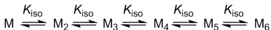
Scheme 2-1. Formation of rosette M_6 by isodesmic assembly of monomer M with K_{iso} .
