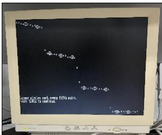
Figure K-3 A photo displaying the time dependent of the value of thermistor. The first and third steps indicate the temperature traces by calibration heating before and after the titration. The second shows an exotherm by the titration.
