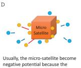
Usually, the micro-satellite become negative potential because the electron speed is faster than the ion speed.
