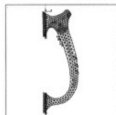
a) Finite Element Model of the grip
