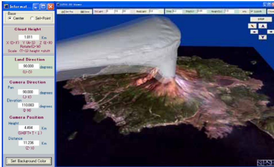
Fig. 6. A model of eruption cloud as a 3D object embedded in a SiPSE 3D image of Sakurajima volcano. The box of parameter control buttons is shown on the left hand side.
