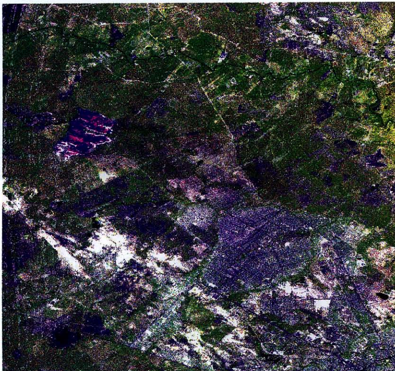
Fig. 3: Large fire near Cuiaba on Aug. 25, 1995 taken from the ER-2 AVIRIS instrument during the SCAR-B experiment. The image is 10x20 km and 20 m resolution. Top image - heavy smoke emitted from the fire and flowing over Cuiaba. The image resembles human vision and is composed of 0.47 \mu\text{m} (blue), 0.55 \mu\text{m} (green) and 0.66 \mu\text{m} (red). Bottom image - is for 2.1 \mu\text{m} (blue), 1.2 \mu\text{m} (green) and 1.65 \mu\text{m} (red). The smoke is almost transparent in these longer wavelengths and the fire is clearly seen with its 3 main temperatures zones (blue - glowing, purple - smoldering - emitting the heavy smoke, and white - the fire front. Note that it is much easier to observe the surface features in the long wavelengths that penetrates the smoke. The solar zenith angle is 36°. The AVIRIS data were provided by Robert Green from JPL.
