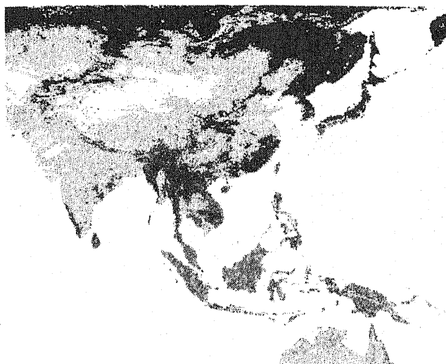
Figure 1 Current land cover. Grey level(0-255) denotes the vegetation/land cover classes. FND(32), FDB(64), FEB(96), FST(128), FTS(160), FTR(192), FBS(208), AGR/GRS(224), SEA(240) and DES(255).
