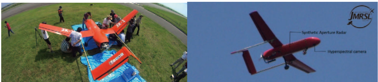
図 1.1.1.-2. CP-SAR ground test of Josaphat Laboratory Unmanned Aerial Vehicle (JX-1) at Fujikawa Airport on 29 August 2013.
