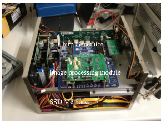
図 1.1.1-9. Chirp Pulse Generator and Image Processing module
