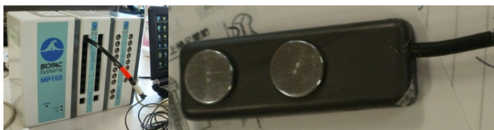
Figure 2-8. MP 150 system (left) and TSD 150A surface EMG electrode (right)
