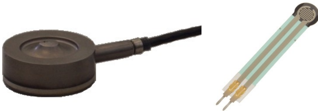
Figure 2-4. Left picture: Load cell (Kyowa Corp., Japan); right picture: pressure sensor (Interlink electronics, USA).
