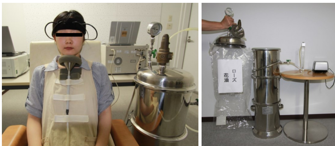
Fig.1 The scene during olfactory stimulation and the device used to administer the odors.
