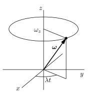
$$\boldsymbol{L} = I_0 \left( \omega_x \boldsymbol{e}_x + \omega_y \boldsymbol{e}_y \right) + I_z \omega_z \boldsymbol{e}_z = I_0 \omega_0 \left( \cos(\lambda t + \theta) \boldsymbol{e}_x + \sin(\lambda t + \theta) \boldsymbol{e}_y \right) + I_z \omega_z \boldsymbol{e}_z$$
