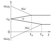
$$t_u = \frac{k}{1+k} \frac{|u_0|}{\mu' g}, \qquad v(t_u) = \frac{v_0 + a\omega_0 k}{1+k} = \frac{\varepsilon}{1+k} v_0$$
