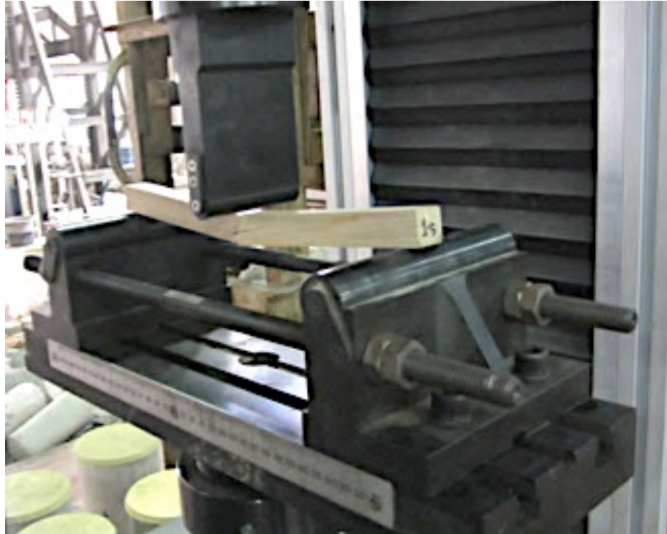
Figure 4.2 The teak specimen was testing of the static bending by the Universal Testing Machine (UTM).
