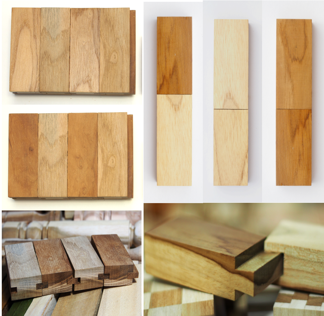
Figure 5.10. Application of parallel-sections (transverse surface) for tongue-and-groove (left side) and dovetail (right side) wood joint system for getting the different color combination of surface appearance
