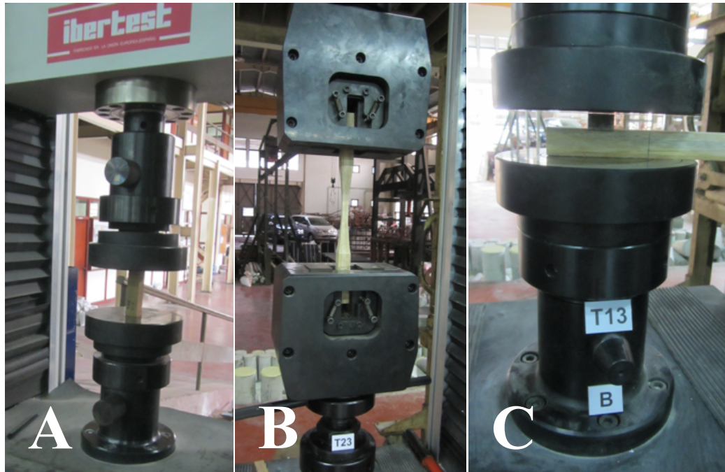
Figure 4.7. Compression (A) and tension (B) parallel to grain, and compression perpendicular to grain (C) tests assembly
