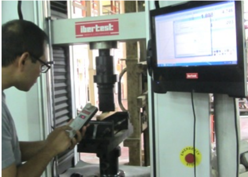
Figure 4.1. The monitor display in UTM shows the increasing loads of pressure to the specimen during the test.
