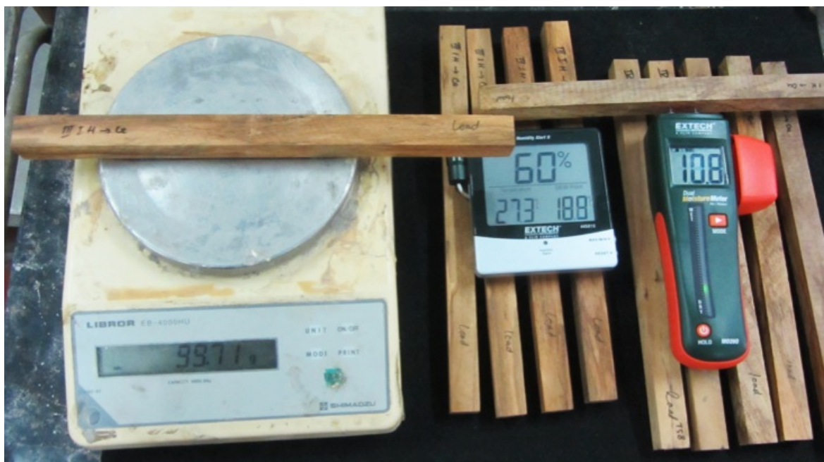
Figure 4.3. Tools for checking the weight and the moisture content of the specimen, the humidity and the temperature of testing area.
