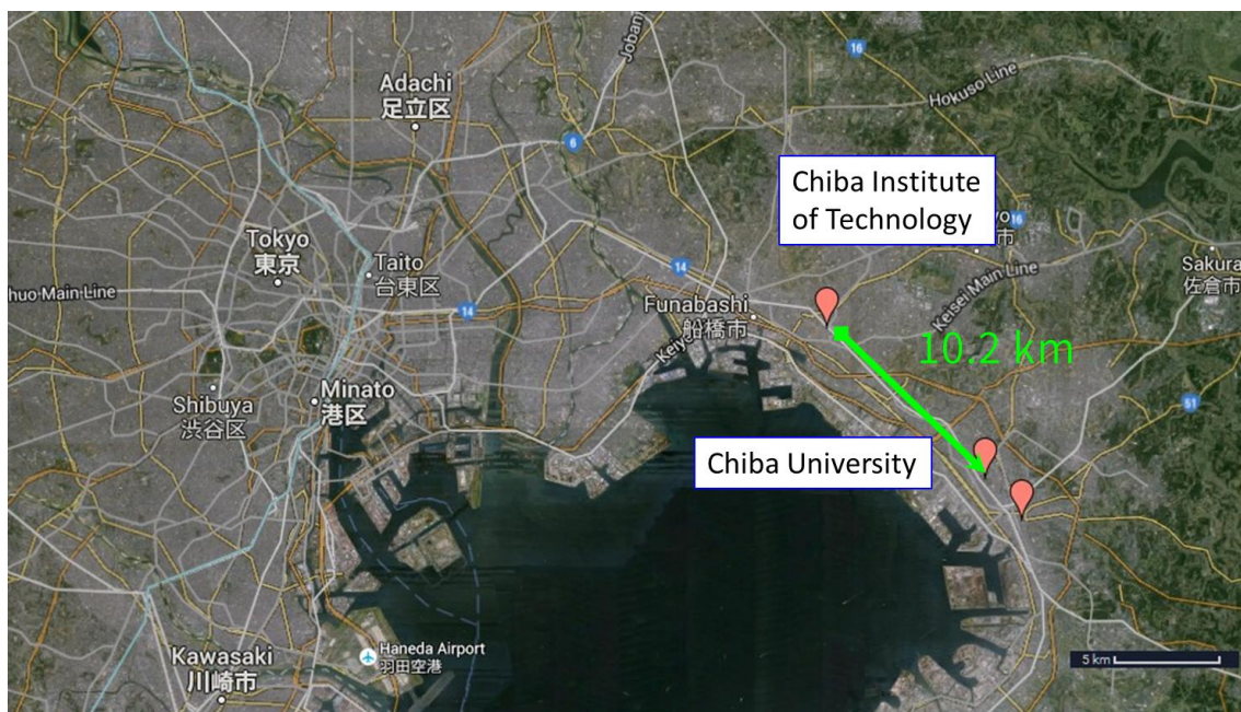
Figure 7.5. The DOAS optical path between Chiba Institute of Technology and Chiba University, with the path length of 10.2 km.
