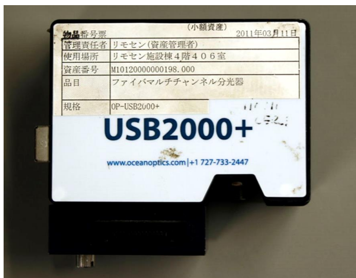
Figure 6.5. The appearance of USB2000 spectrometer. The instrument is controlled by a PC via USB interface.
