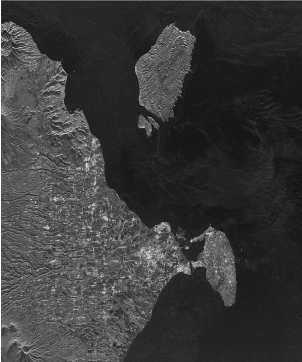
Figure 4.2: Intensity image of JERS-1 SAR sample data used for the experiment if processed with Range Doppler Algorithm (3 Looks)
