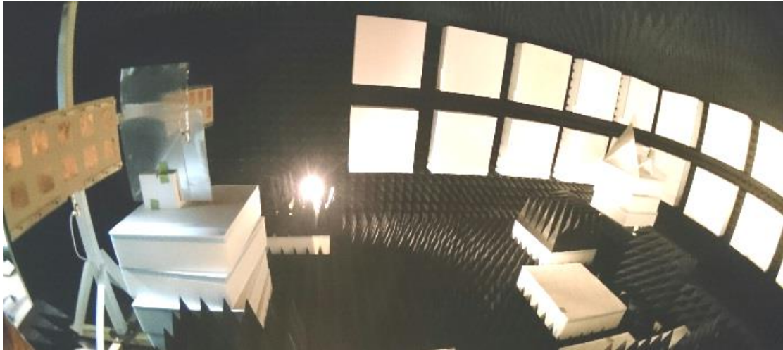
Figure 5.1: The reduced side-lobe antennas installed on the mounting on the left and corner reflector placed on the moving platform on the far right of the image.
