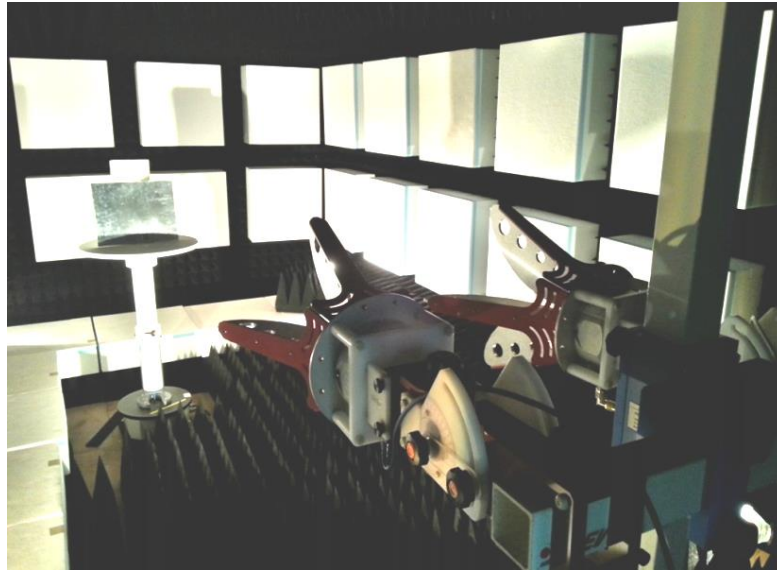
(a) Metal plate for point target measurement placed on a rotating polystyrene platform in an anechoic chamber. Note the quasi-monostatic placement of the receiving and transmitting horn antennas.
