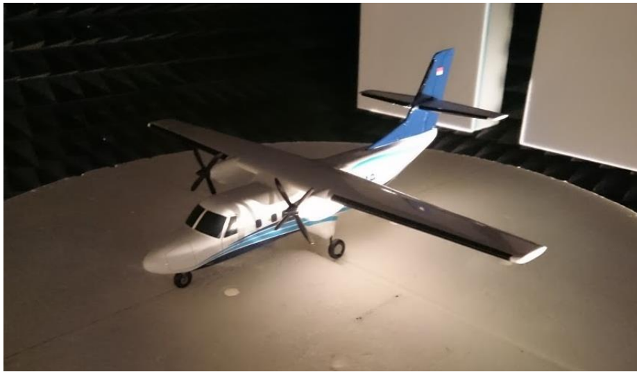
Figure 5.18: A model airplane used a complex target to be imaged by the developed system.
