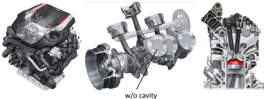
Fig.1.12 Stratified mixture formation control using spray guide (53) (Audi)
