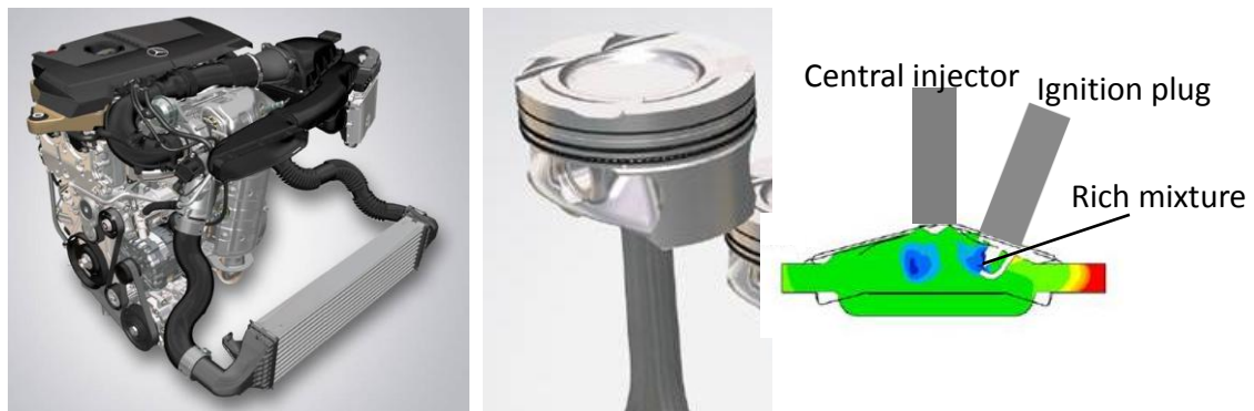
Fig.1.11 Stratified mixture formation control using spray guide (52) (Daimler)
