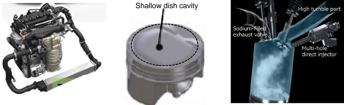
Fig.1.8 Stratified mixture formation control using wall guide (49) (Honda)
