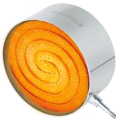
Fig. 1.20 Electrically heated catalyst (111) (Continental: The EMITEC®)
