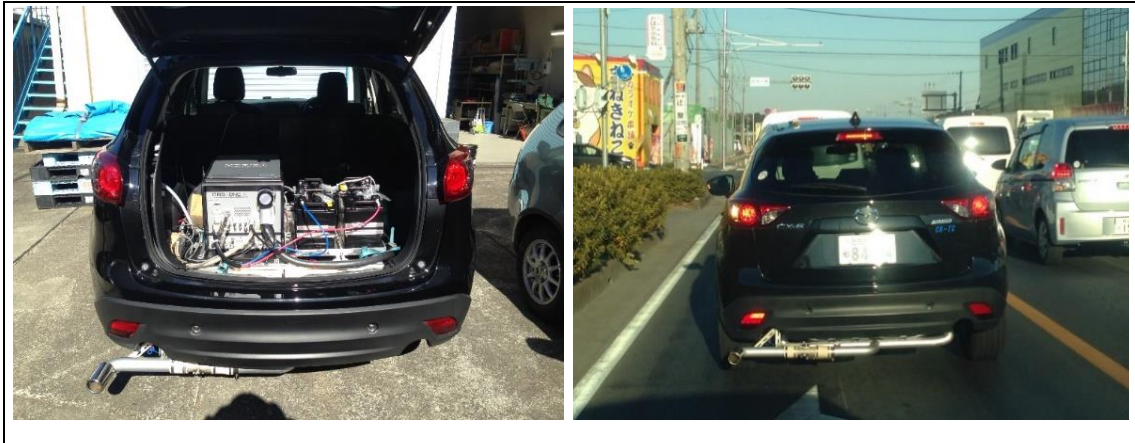
Fig.3.2 Schematic of measurement system using PEMS
