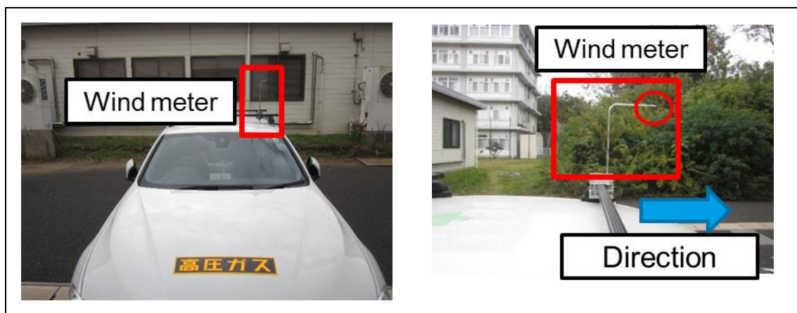
Fig.5.2 Photo of wind meter
