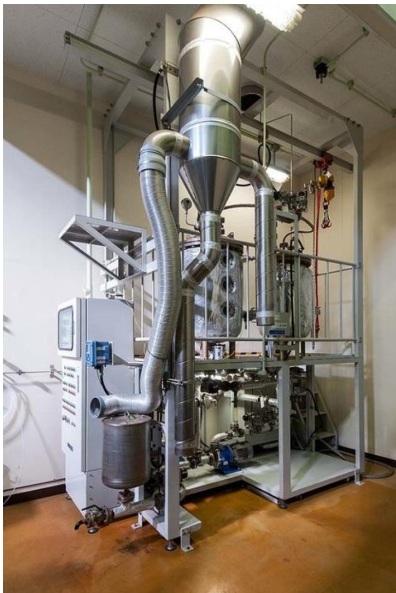
Fig. 6-7 Graft polymerization apparatus
