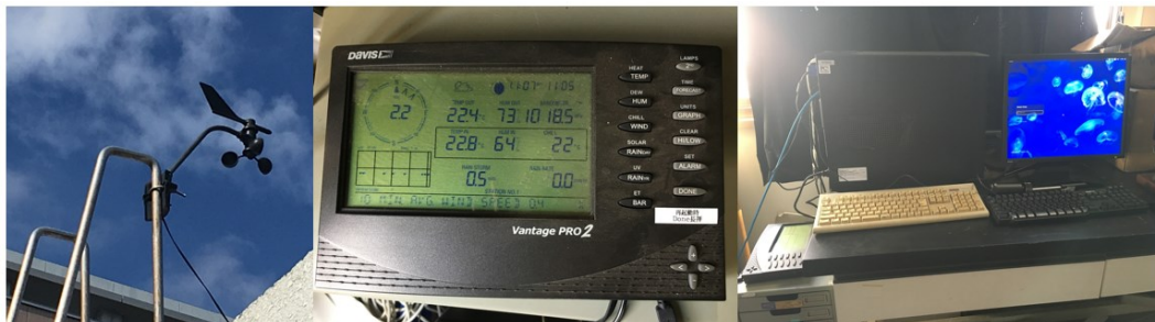
Figure 3.3: Weather monitor installed in CEReS-Chiba University for monitoring the temporal change of ambient RH, temperature, air pressure, wind speed, and wind direction.
