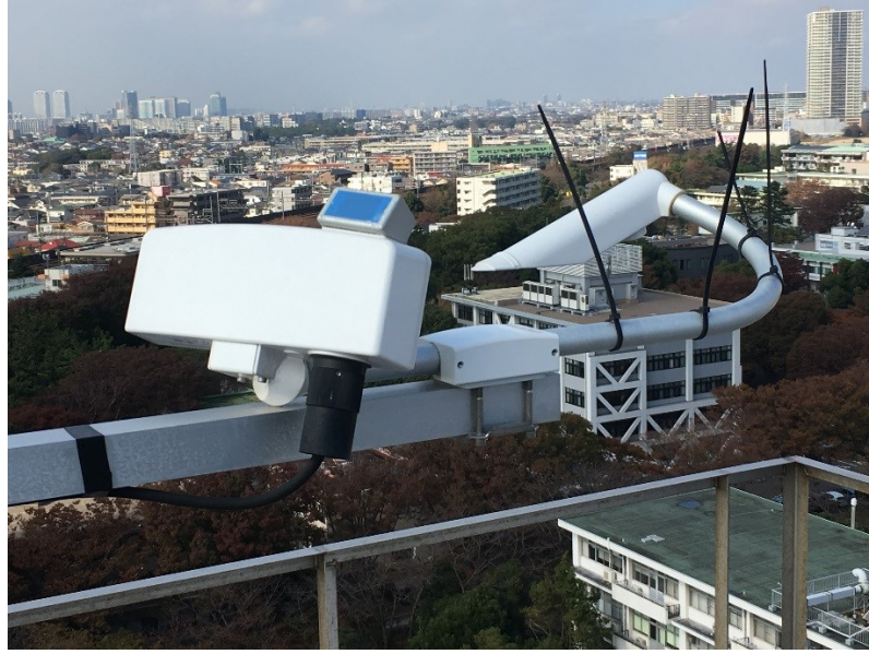
Figure 3.22: The visibility-meter with the wavelength 550 nm installed on the 9th floor of engineering building.
