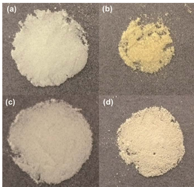
Figure 25. Sample appearances of (a-b) LVFX·½H 2 O and (c-d) LVFX-AMAP co-crystal. (a, c) and (b, d) is the samples before and after irradiation 1.2 million lx·h, respectively.
