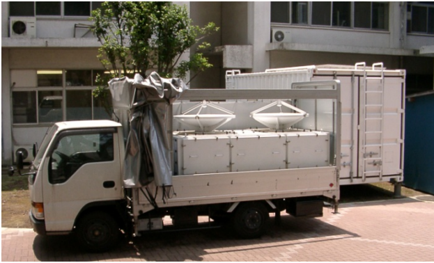
Fig.2. FALCON-I installed on a truck in the campus of Chiba University. The container behind the truck is housing of FALCON-I with two Teflon sheet windows on the ceiling for MIRAI observations (see Fig.4).
