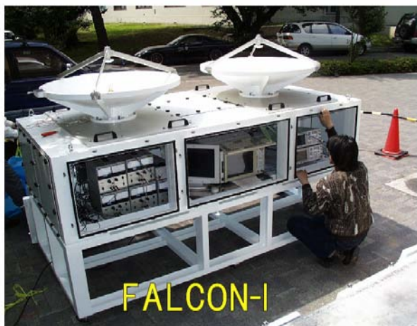
Fig.1. Cloud profiling radar FALCON-I. It has two 1-m diameter antennas which transmit and receive radio waves at 95 GHz.
