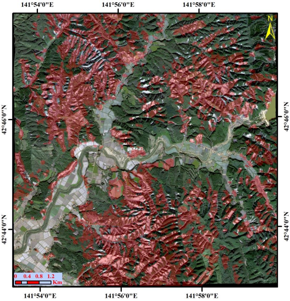
Figure 5.13 The landslide classification map using coherence difference in both descending and ascending SAR images. The background image is a high-resolution GeoEye-1 image taken on 20 October 2018.
