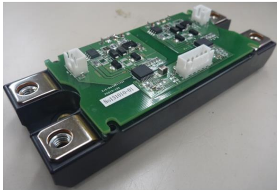
SiC Module BSM120D12P2C005(ROHM, 1200 V / 120 A)
