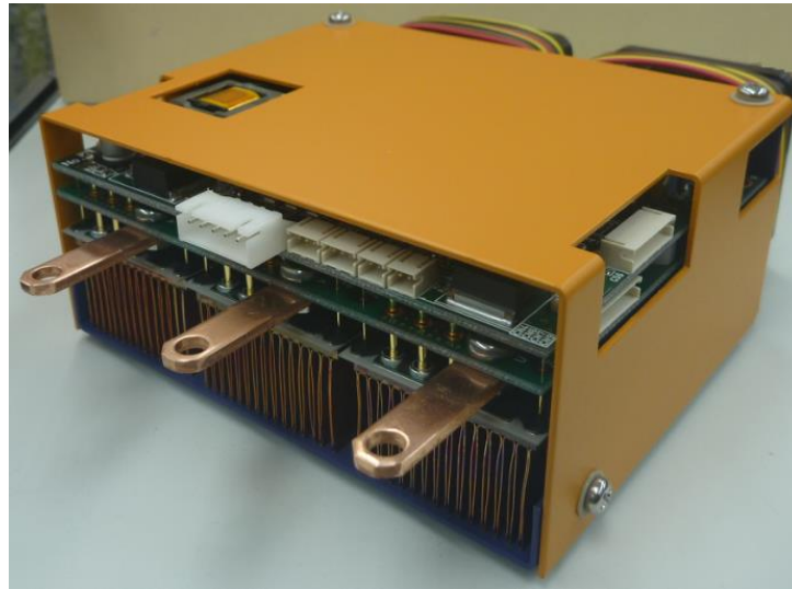
(a) External view of inverter.
