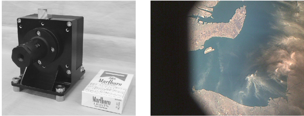
Figure 2.1-9. Overview of the two-dimensional complementary metal oxide semiconductor image sensor (CMOS) camera (CAM) and an image captured near Nagoya, Japan (image credit: JAXA).
