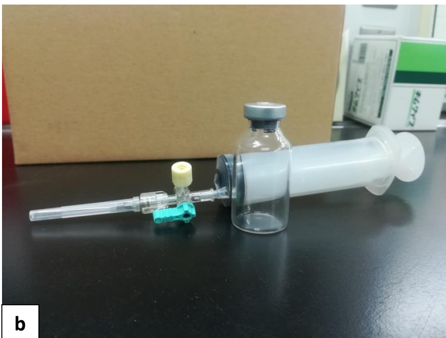
Plate 2-1: Preparation of evacuated glass vials. (a) = a glass vial, butyl rubber stopper, and aluminum cap and (b) = a prepared glass vial for gas sampling.
