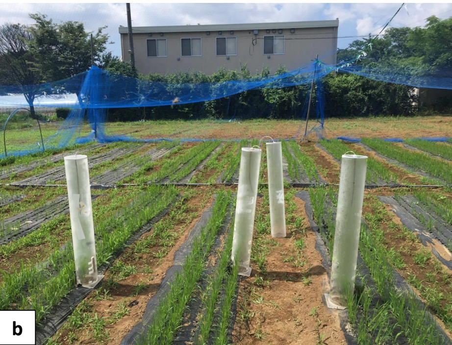
Plate 2-3: Gas sampling using close chamber method. (a) = continuous flooded system and (b) = drip irrigation with plastic-film-mulch system
