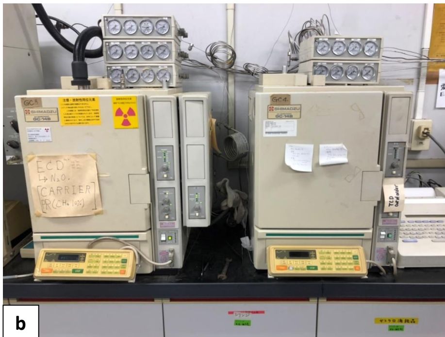
Plate 2-4: Preparation of a standard gas and sample analyses. (a) = prepared standard gas and (b) = Gas chromatograph with a flame ionization detector (FID) for CH 4 and Electron Capture Detector (ECD) for N 2 O.
