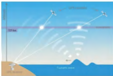
➤ Figure 2. Sea surface disturbances induced by tsunami propagate into ionosphere, while a ground-based GNSS receiving station monitors ionospheric disturbances. The thin-shell ionospheric (i.e. ionospheric pierce or ionospheric) height is at 325 km altitude.
