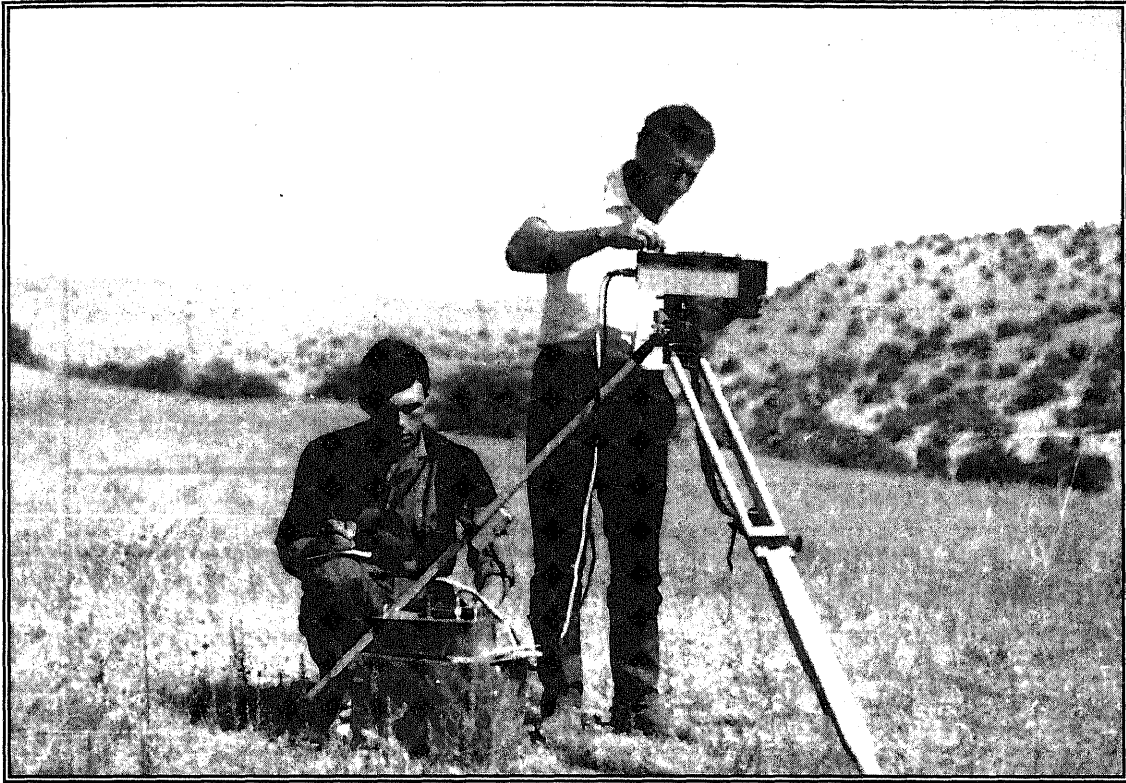
Figure 3.3.4. Measurement of spectral reflectance coefficients in the field.
