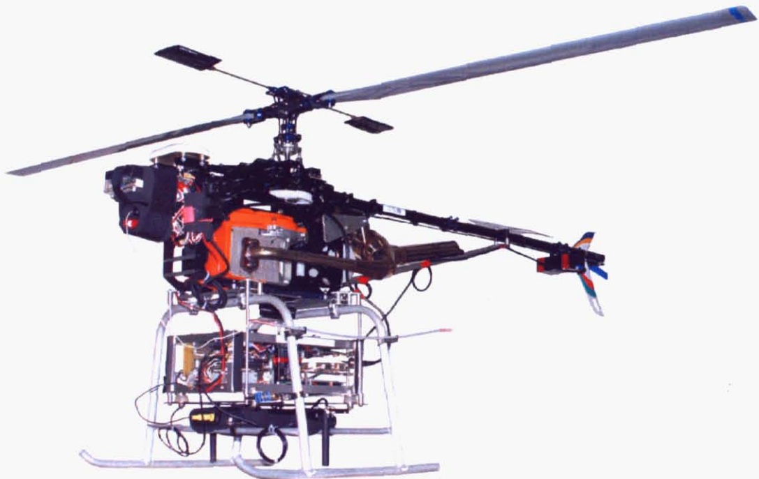
Fig. 2.1: HIROBO SF40 with equipments for the autonomous control
