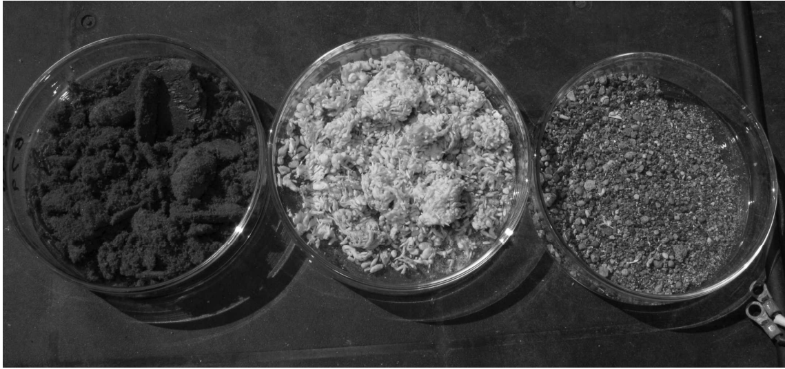
Photo 13 Substrates used for the experiment, foam phenolic resin (left), rockwool (middle) and river sand (right)
