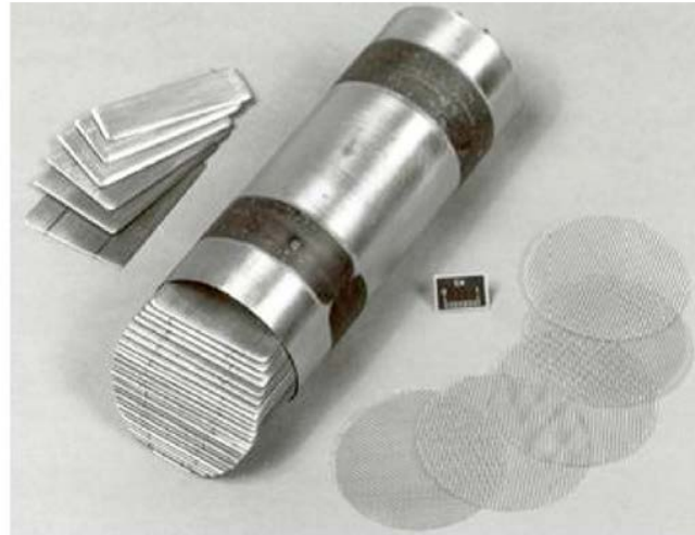
Figure 1-1: First room-temperature magnetic heat pump designed by G. V. Brown [3]
