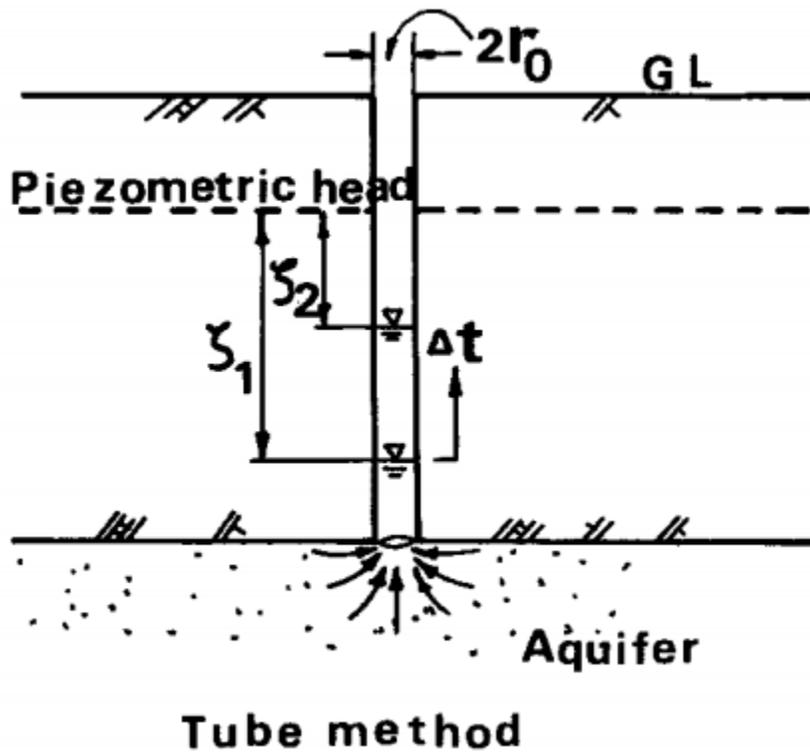
Figure 3- 3 Tube method-slug test
