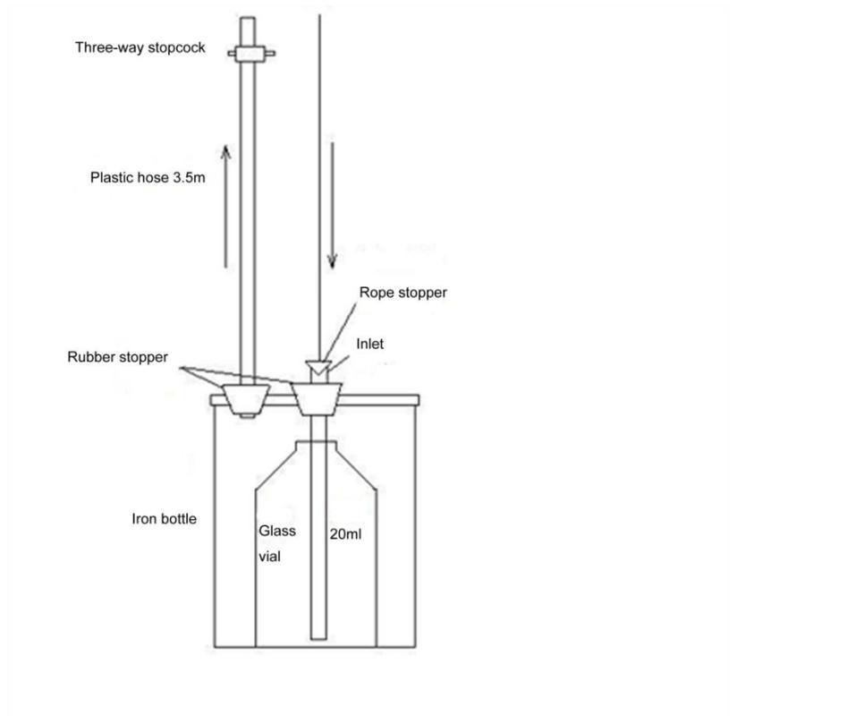
Figure 2-3 The Schematic diagram of sampler for dissolved  $N_2O$
