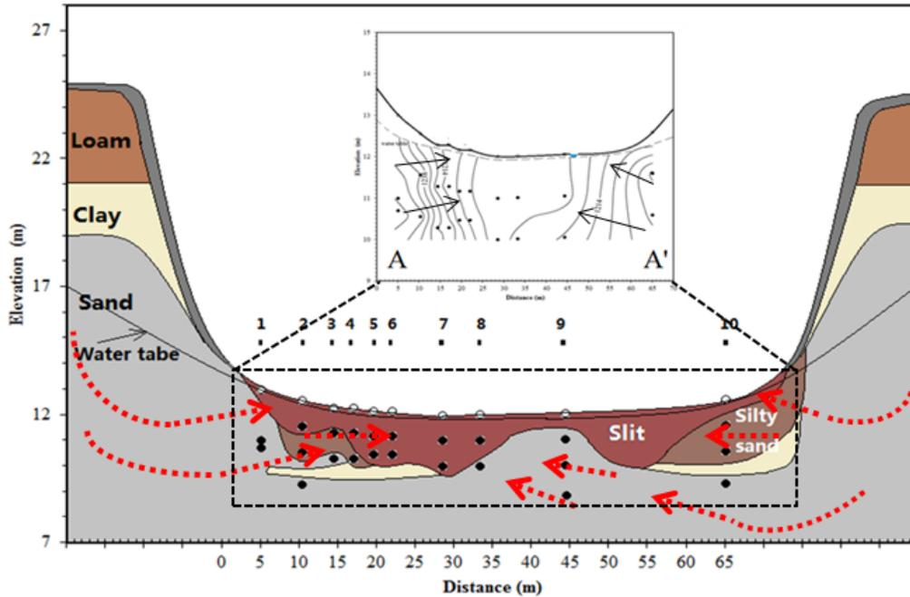
Figure 3-6 Piezometers nest and hydraulic head contours along cross section A-A'. The arrows present the direction of flow path.
