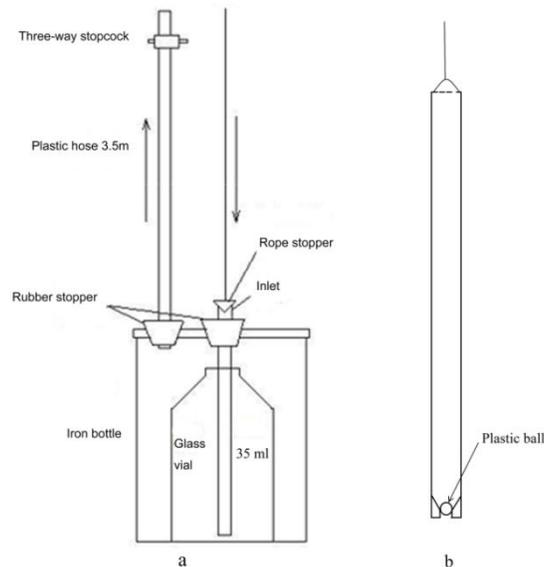
Figure 5- 2The schematic diagram of sampler for dissolved  $\text{N}_2\text{O}$  (a) and ion, parameters and  $\delta^{15}\text{N-NO}_3^-$  (b)
