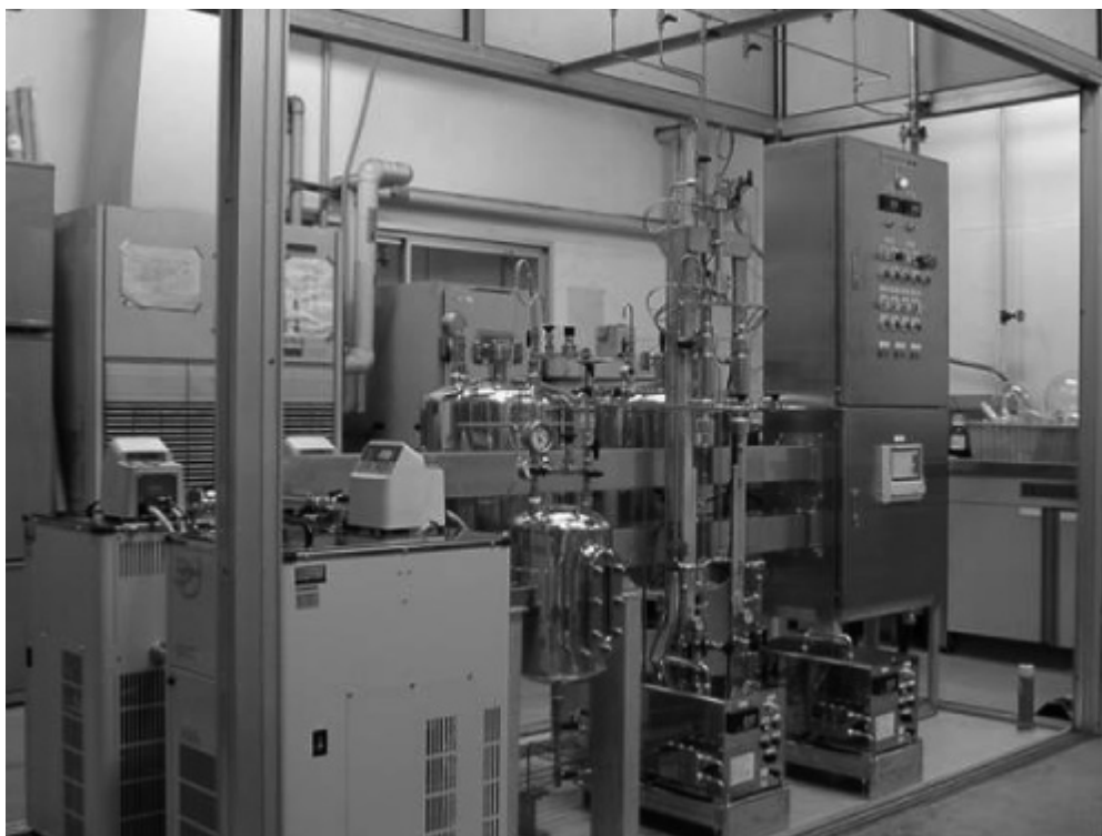
Figure 5. Picture of the Pilot Plant for the Reaction of 12 with 13 7
