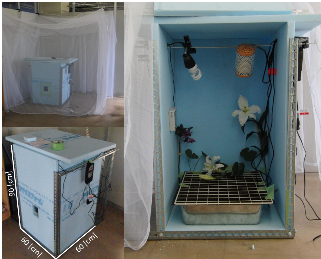
Fig. 3.1 Glass house with the thermostat for keeping adult moths.
