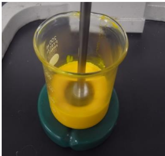
Fig. 4. Photographic Image of Riboflavin Suspension during Bead Milling
