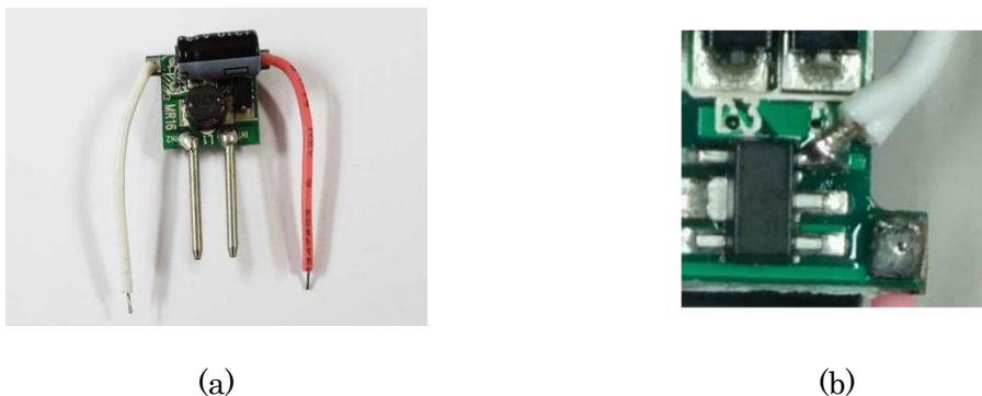
Figure 2.5: Constant current high power LED driver: (a) overview of the driver, and (b) additional processing for the driver.
