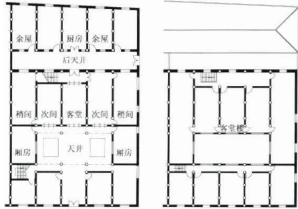
Figure 3.4 Xingren Li, a five-room traditional shikumen houses, built in 1872 (from Wang 1987, 7)
