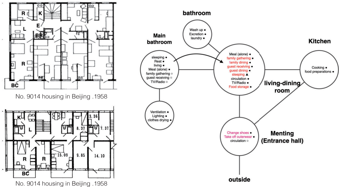
Figure 3.48 Late Ting type housing and domestic code < 5 >
