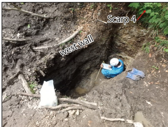
c Portable percussion coring at the Wakamaru-yama site
