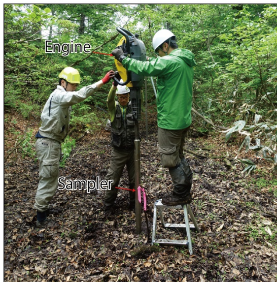
Fig. 3-2. Photographs showing field methods and equipment of this study. (a) Hand coring at the Wakamaru-yama site. (b) Pit excavation at the Wakamaru-yama site. (c) Percussion coring at the Wakamaru-yama site. (d) Sampler and linear-tube of the PPCS. (e) Bit and core-catcher at the tip of the sampler.
