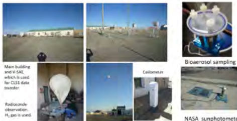
Dalanzadgad observatory is located in the Gobi Desert. Installed are radiosonde by China, a collimator by Nagoya University, a sunphotometer by NASA, a bioaerosol sampler by Kanazawa University.
