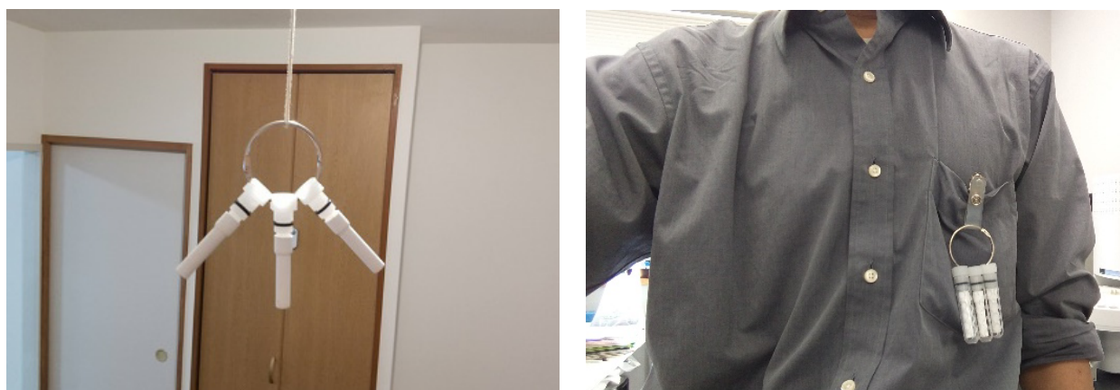
Fig. 5-2. Collection of gaseous chemical compounds in indoor air (left panel) and personal exposure (right panel) using three kinds of DSD samplers.
