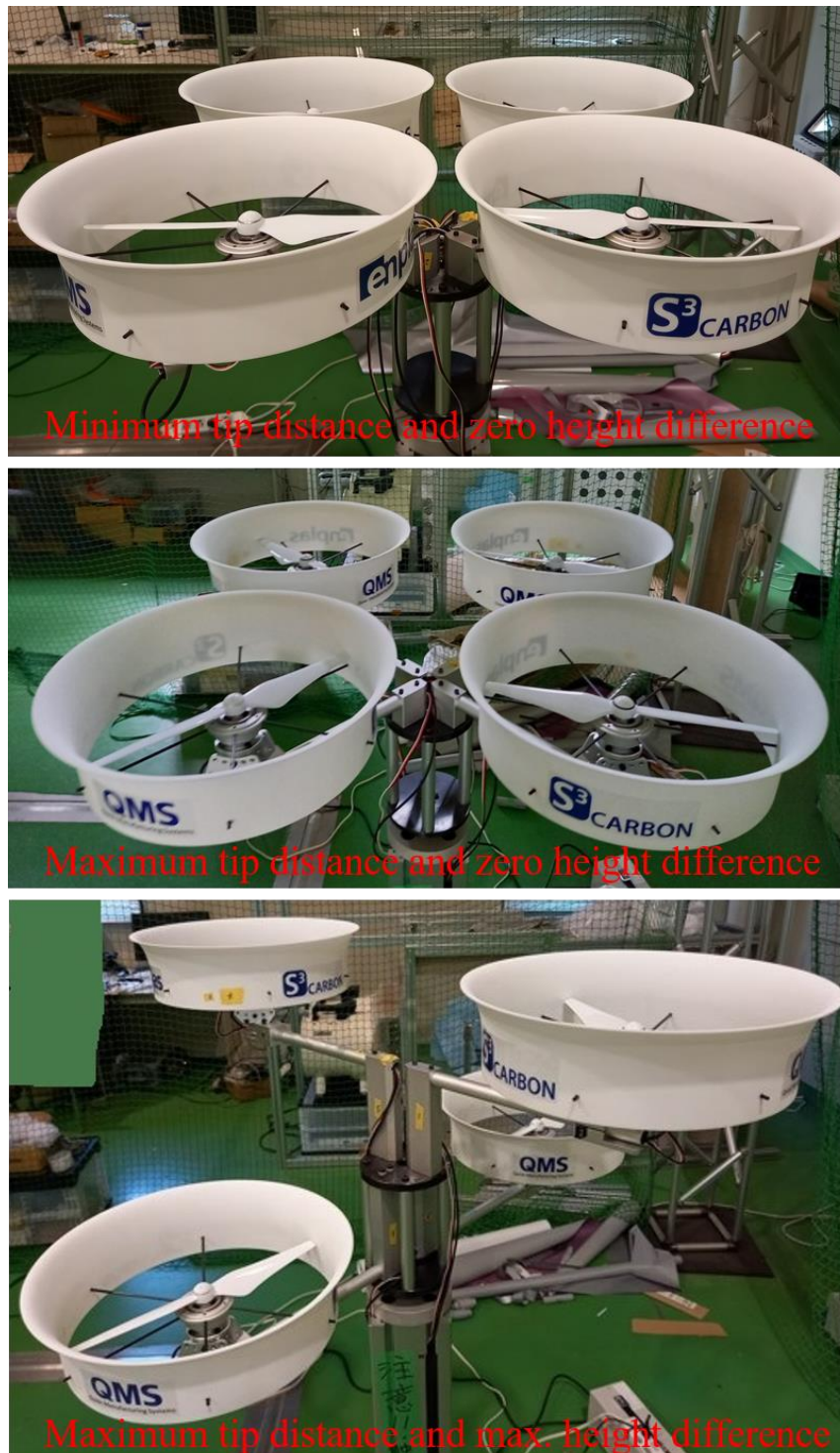
Figure 4-11 Illustration of different cases regarding ducted rotor-configurations in the experiment.
