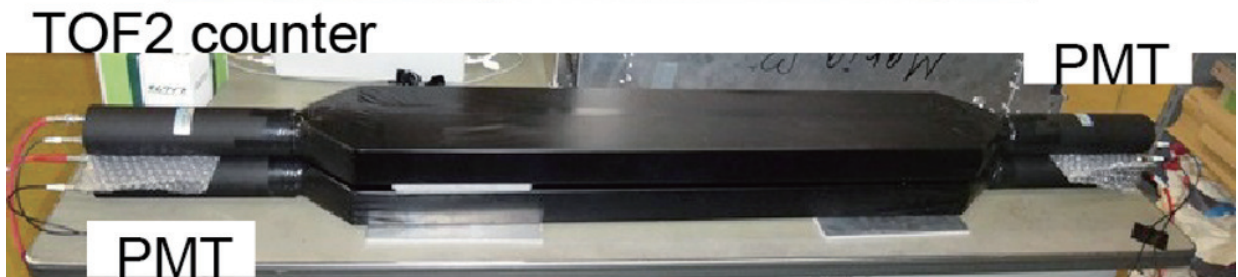
Figure 20: The TOF2 counter. The counter size was 800 \times 200 \text{ mm}^2 and 200 mm, which was located about 90 cm behind C4 resulting in a typical path length of 2.7 m from TOF1.
