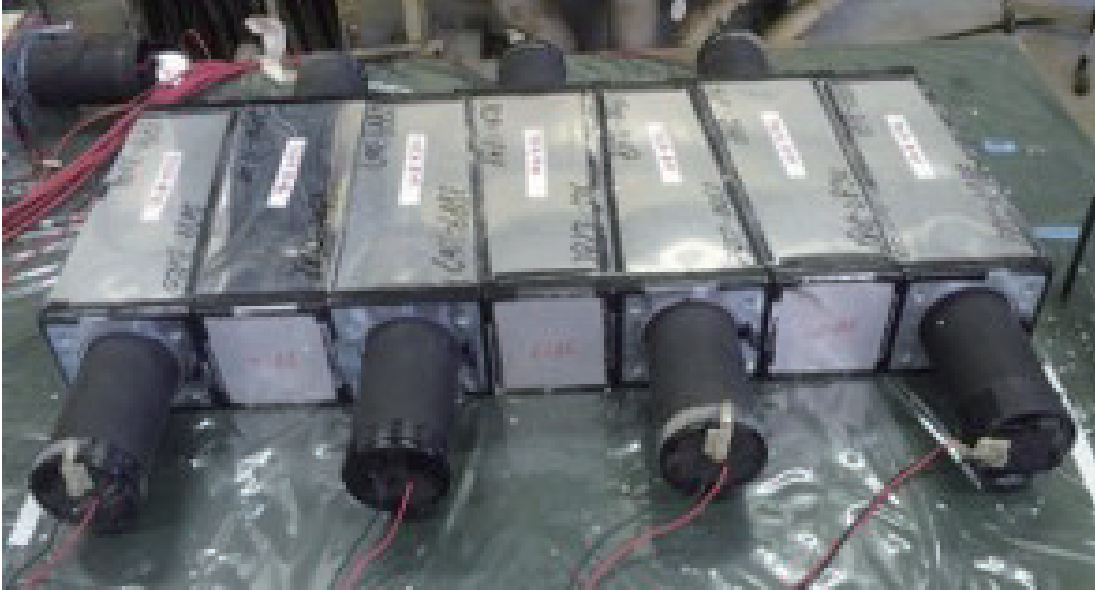
Figure 22: The PGC system was assembled with 7 lead-glass modules stacked in a radial direction behind the TOF2 counters. A polyethylene degrader of 10 cm in front of the PGC slowed down the charge particle momentum and improved the PGC performance as a PID detector
