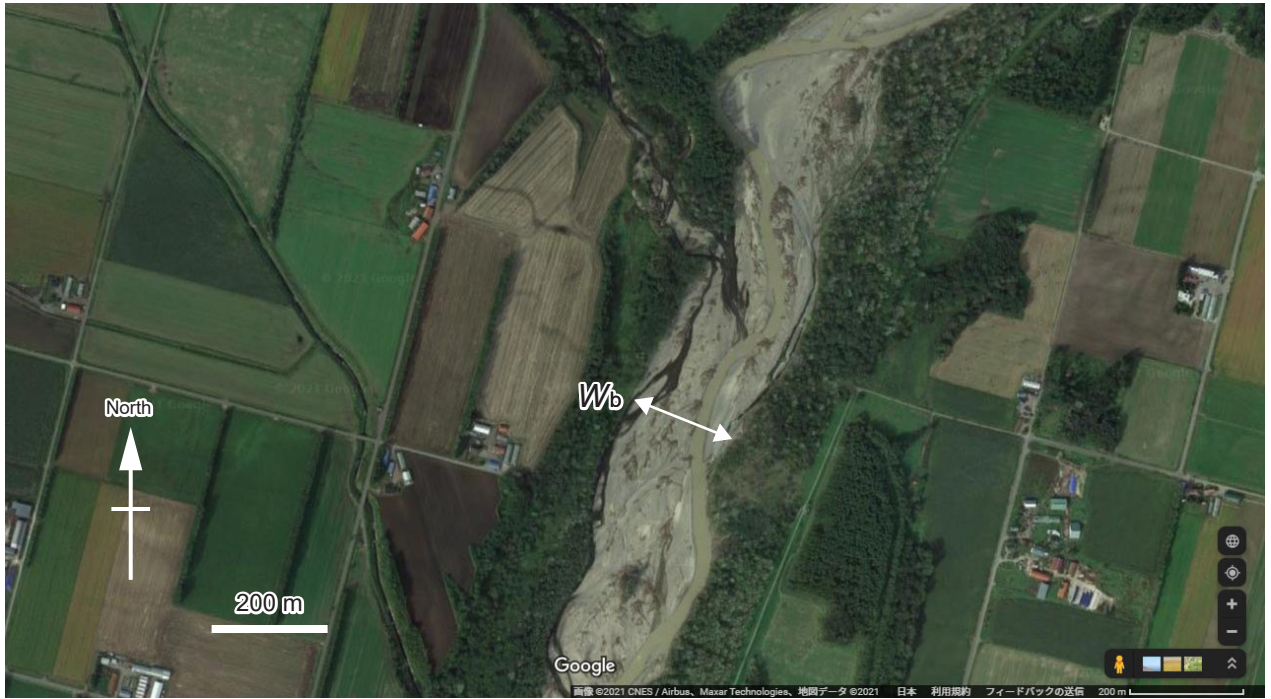
Fig. 8. Measurement of a bankfull channel width ( W_b ) from an aerial photograph (Google Map: https://www.google.co.jp/maps ). The examined river is the Otofuke River near Shihoro, Hokkaido ( 43^{\circ}11'11.5''N , 143^{\circ}13'20.1''E ) (site 35 in Fig. 4 and Table 1).
