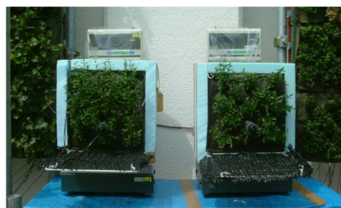
Photo.2 The measurement situation of quantity of evapotranspiration using electronic scales
