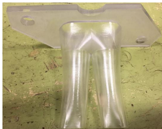
Figure 4-4 high tumble generation nozzle
