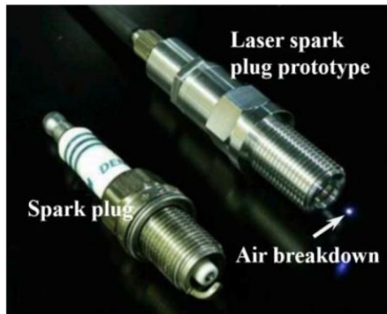
Figure 1-12 Comparison of laser ignition and traditional spark plugs [59]
