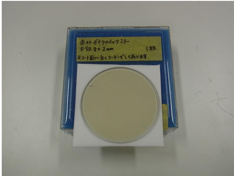
Figure 2-17 The special infrared dichroic mirror
