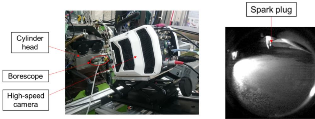
Figure 1-28 Experimental setup and the view of the in-cylinder around the spark plug. [91]
