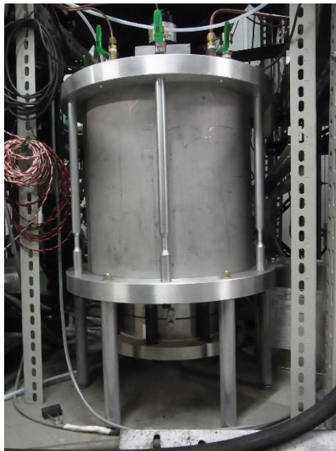
Figure 2-8 The gas mixture chamber
