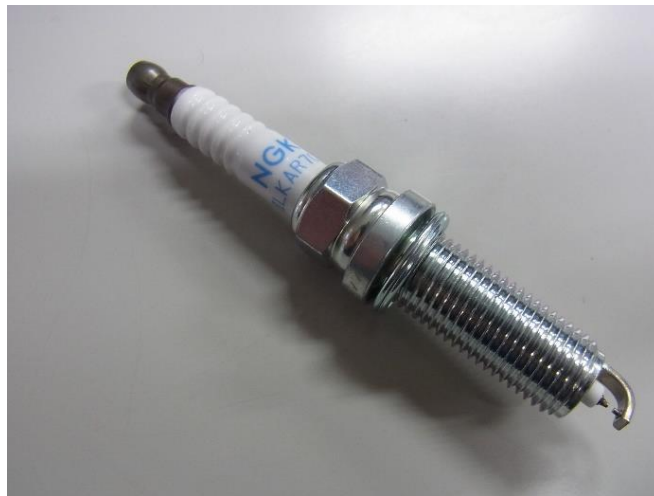
Figure 2-7 Overview of spark plug
