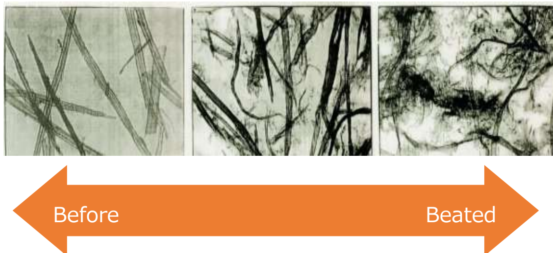
Fig. 2-1 Image of beaten cellulose pulp 1) .
