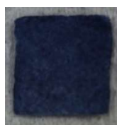
Fig. 3-17 Photograph of a p70/O3MeOT sheet re-doped with 70wt% perchloric acid after nitrogen fixation experiment in N 2 atmosphere.
