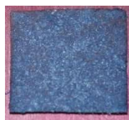
Fig. 3-18 Photograph of a re-doped p70/O3MeOT sheet by diluted perchloric acid solution after the nitrogen fixation experiment in an N 2 atmosphere.
