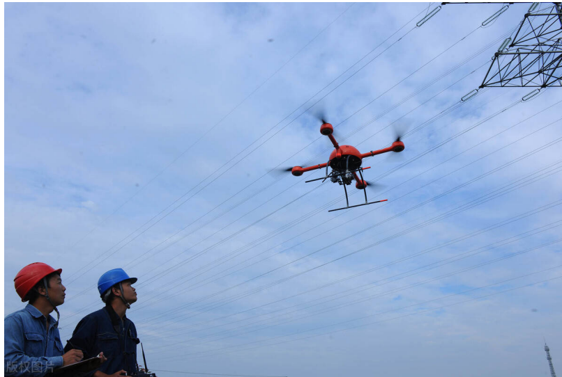
Figure 2-7: UAV transmission line inspection.
