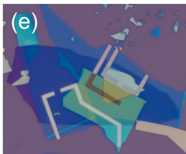
SD electrodes (Cr/Pd) on second h-BN
