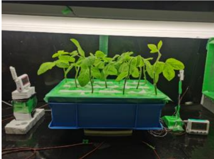
Figure 3.4 A photo of measuring transpiration rate under different inflow parameters (velocities: 0.2–0.8 m s -1 ; temperatures: 23–25 °C; and humidities: 60–70%). The deviation of transpiration was smaller than 6.5% under those conditions.
